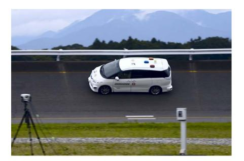
Currently, Bridgestone is conducting various tire performance tests on its proving grounds that involve test drivers operating vehicles. This new joint development project with ZMP is aimed at achieving automated driving for tire noise tests. In this project, ZMP conducts development of technologies for automated driving
